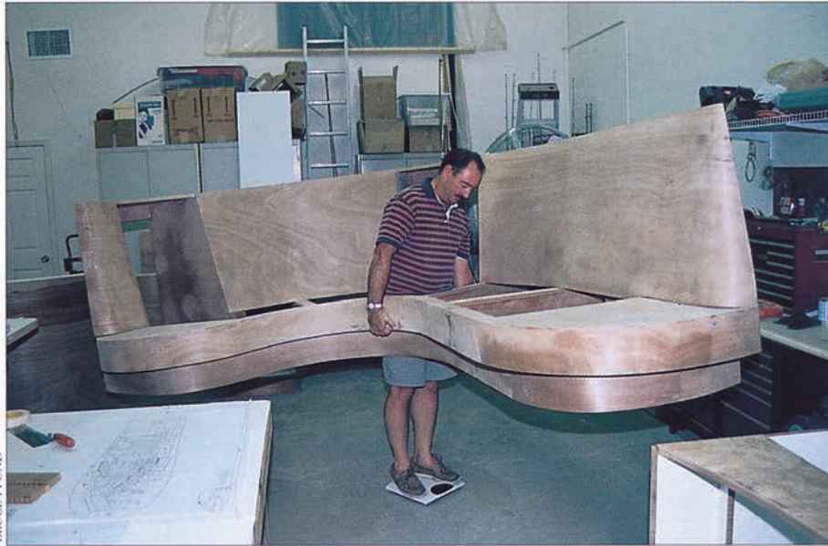
Evans easily hefts an 85-lb (39kg) main-saloon module built of curved honeycomb-cored panels.
