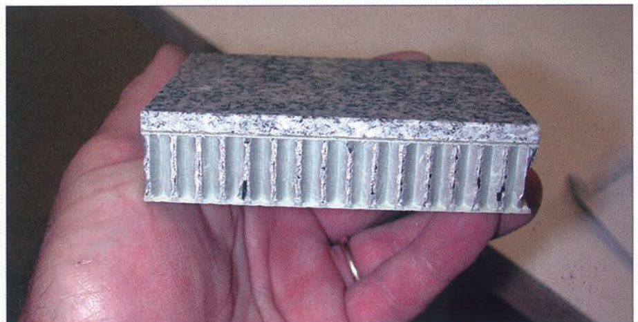
A close look at the marble-faced, aluminum-honeycomb-cored panels that Evans selected for vanity and galley countertop surfaces. The panels will be adhesively bonded to the cabinets underneath.
